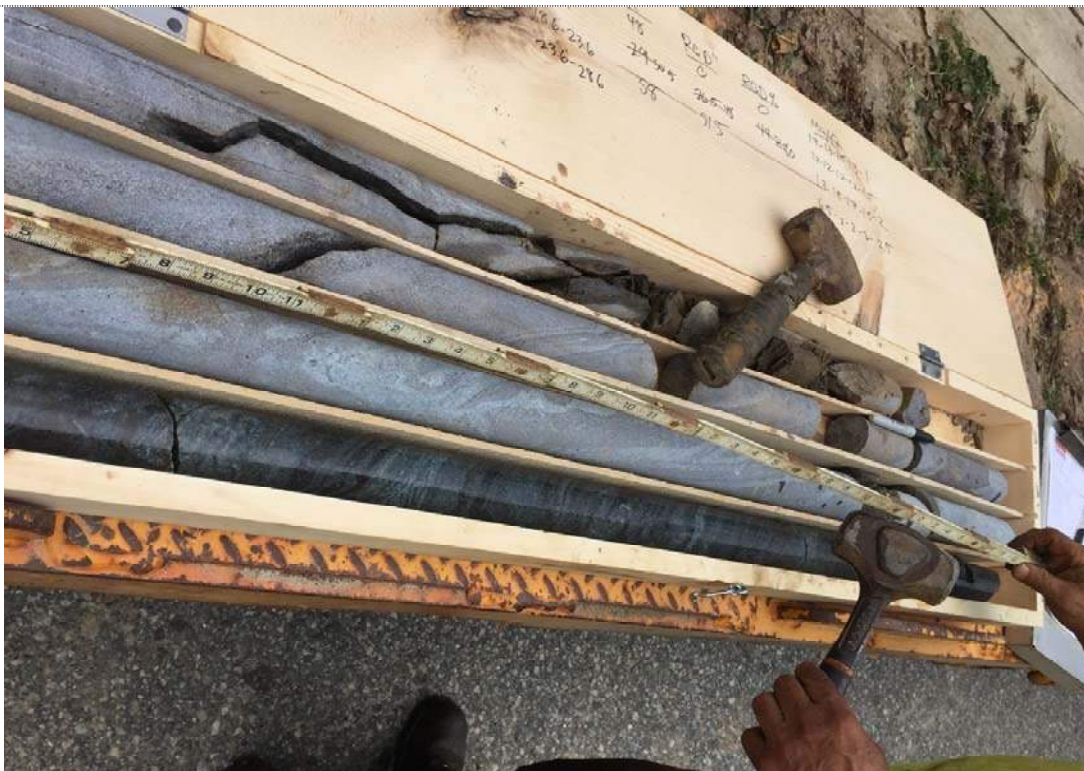
Photo 3: Boring BB-SHEBNR-102 Rock Core Sample R-2 (Row 2, Bottom)
