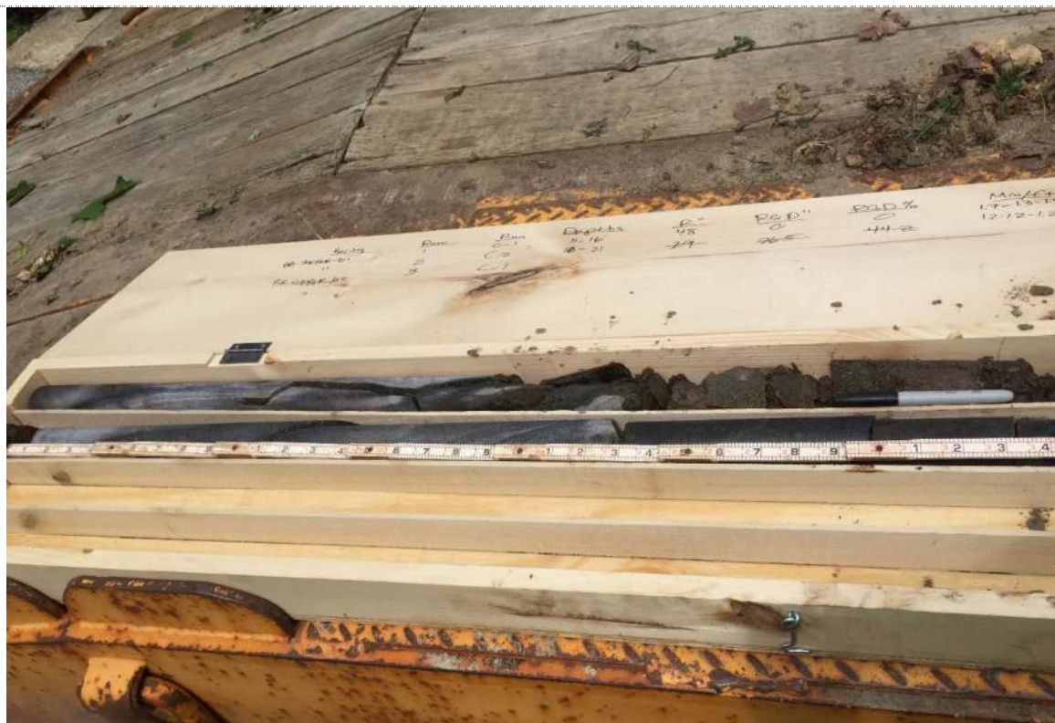
Photo 3: Boring BB-SHEBNR-101 Rock Core Sample R-2 (Row 2, Top)
