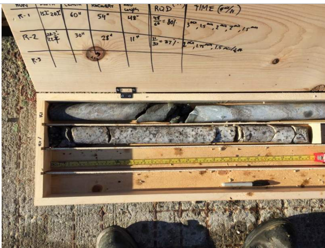
Photo 2: Boring BB-SHEBNR-104 Rock Core Sample R-2 (Row 2)
