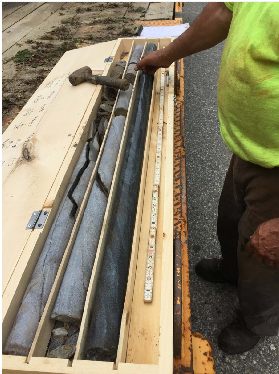
Photo 1: Boring BB-SHEBNR-102 Rock Core Sample R-1 (Row 3)
